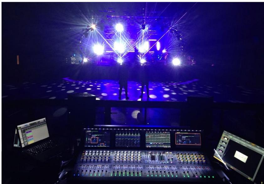
Joining their GLP stable-mates on the tour are 12 GLP impression X4 Bar 20s, a 20 LED batten with a zoom range from 7° to 50°. Novatech have invested heavily in the X4 Bar 20s, with a huge fleet in the warehouse. Their high quality optics ensure smooth, homogenised output through a broad pallet of pastel and saturated colours, while their full DMX control mode offers pixel mapping capabilities, allowing a multitude of dynamic fades and chases through intensities and colours.
